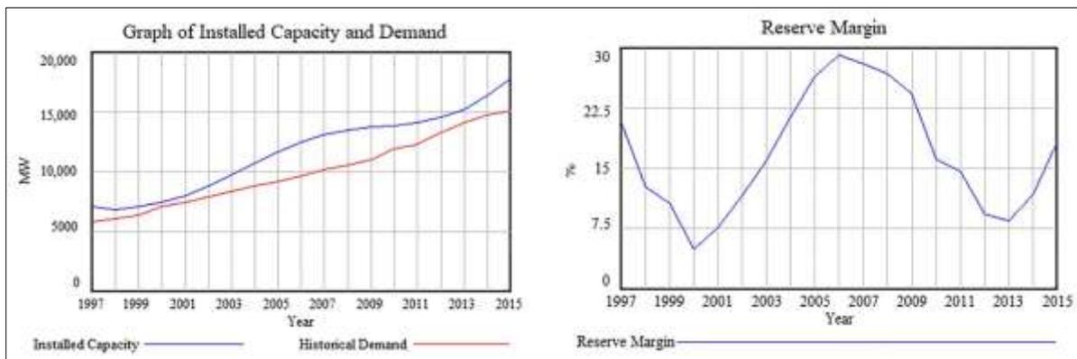
Figure 3. Figure 3(a) Forecasted Demand and Modelled Installed Capacity, (b) Modelled Reserve Margin
