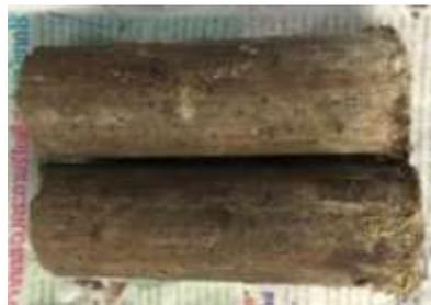
Figure 4. Fuel with High Starch Components from a Ratio of 1:1:1 with a Pressure of 20 kgf/cm<sup>2</sup>
