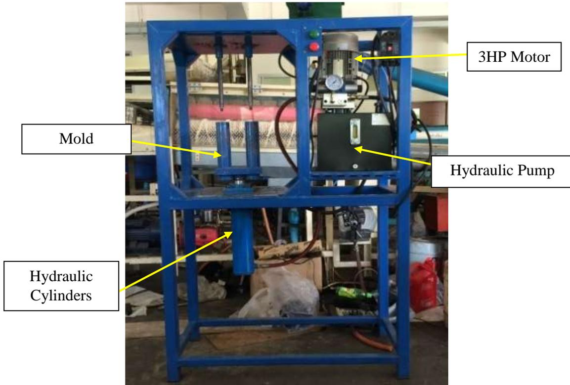
Figure 2. Palm Meal Fuel Briquette Compression Machine
