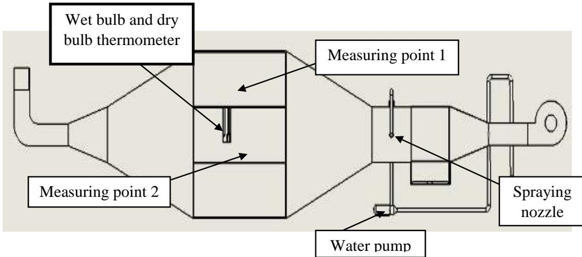
Figure 2 Illustration for the design of development of community palm semi-damp dryer
