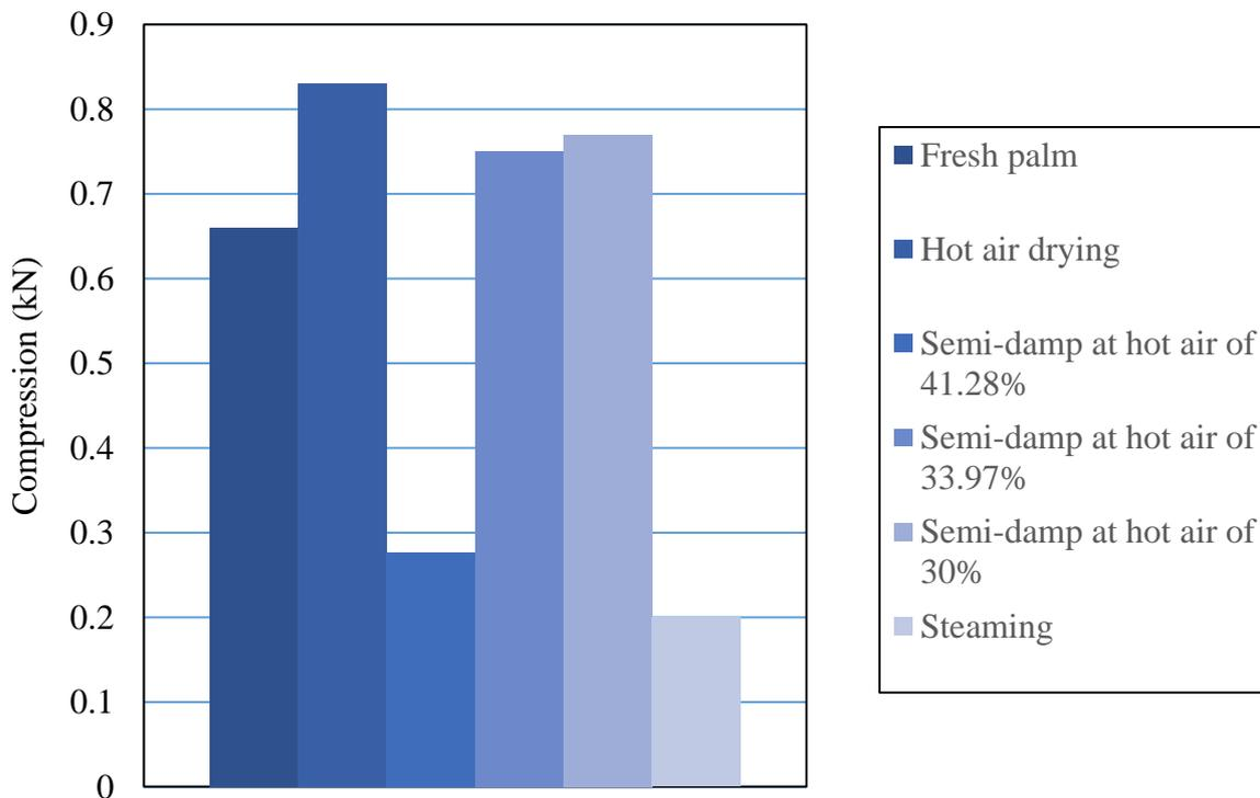
Figure 3. Graph representing the efficiency of palm seed compression test, the temperature in the oven at 70 °C
