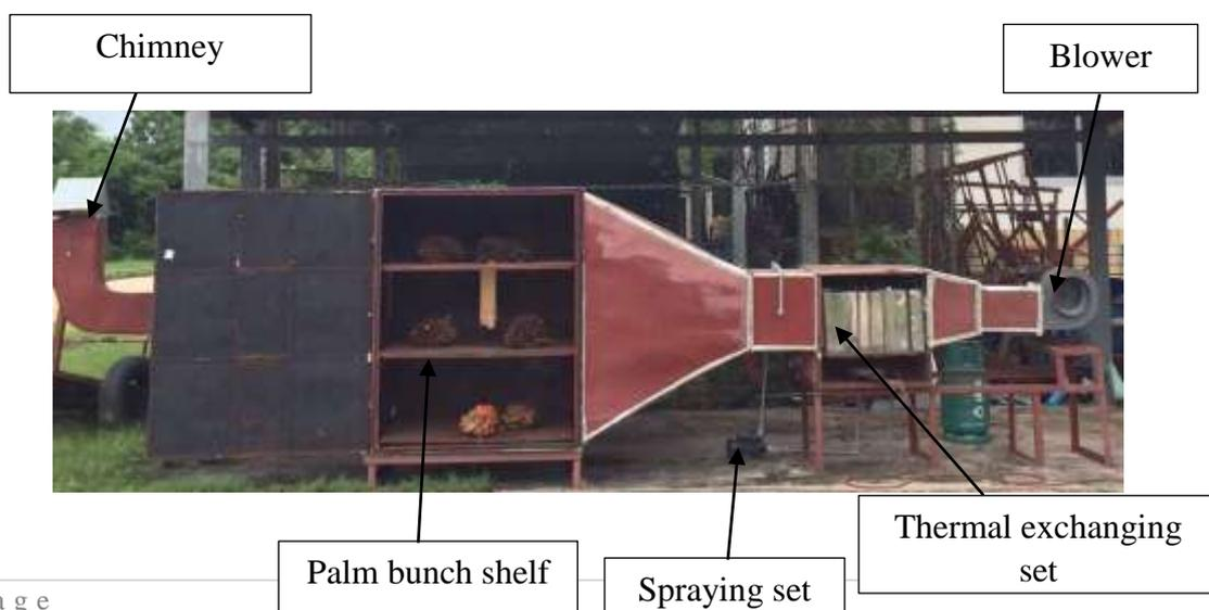
Figure 1. Parts of community palm semi-damp dryer
