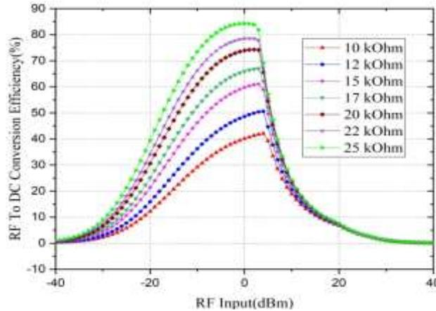
Fig. 9. The dc rectification efficiency for seven different RL values.
