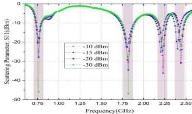
Fig. 7. The simulated, S11 for different ambient power levels.
