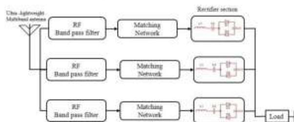
Fig. 3. Block diagram and symbolic schematic of multiband rectifier.
