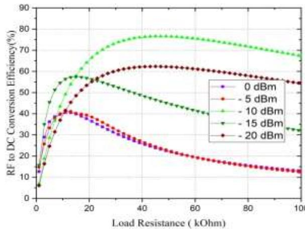
Fig. 8. The simulated conversion efficiency for different load values.
