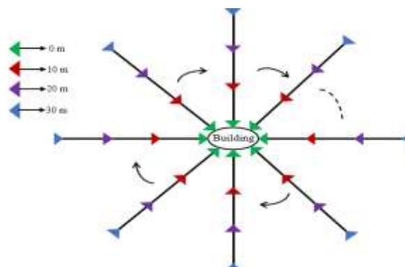
Fig. 1. Procedure for conducting RF spectral survey in each building. Distance is measured in meter (m).
