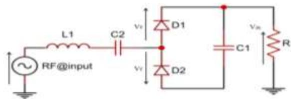
Fig. 4. Schematic view of the proposed rectifier section.
