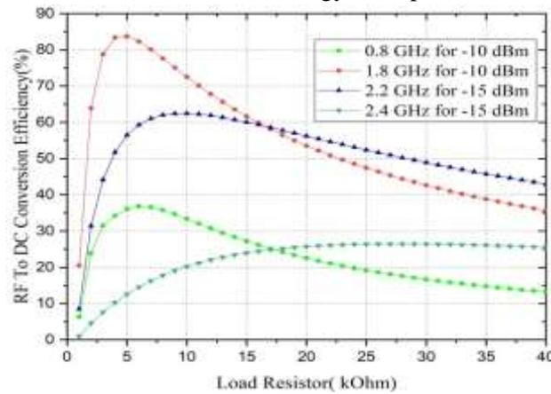
Fig. 10. The dc rectification efficiency for seven different RL values.
