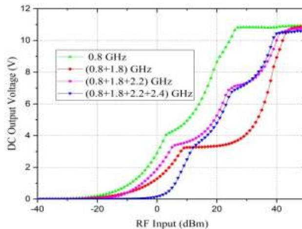
Fig. 11. The Simulated  $V_{dc}$  Value For Different Signal Tones.
