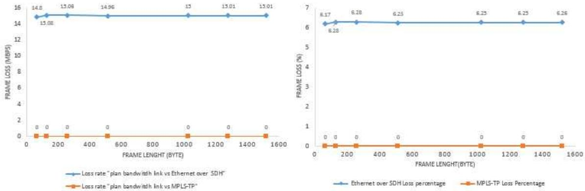
Figure 4. The Value of Frame Loss. (a) The Value of Frame Loss from Actual Link Plan, Ethernet over SDH and MPLS-TP. (b) The Frame Loss in Percentage from Actual Link Plan, Ethernet over SDH and MPLS-TP.
