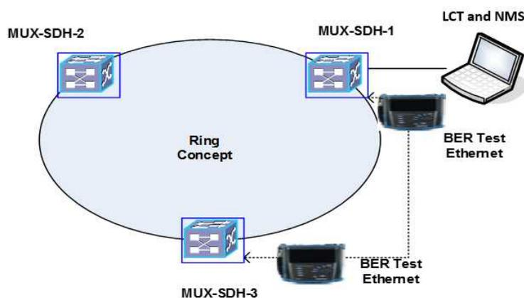
Figure 1. Topology of Ethernet over SDH (EoS)
