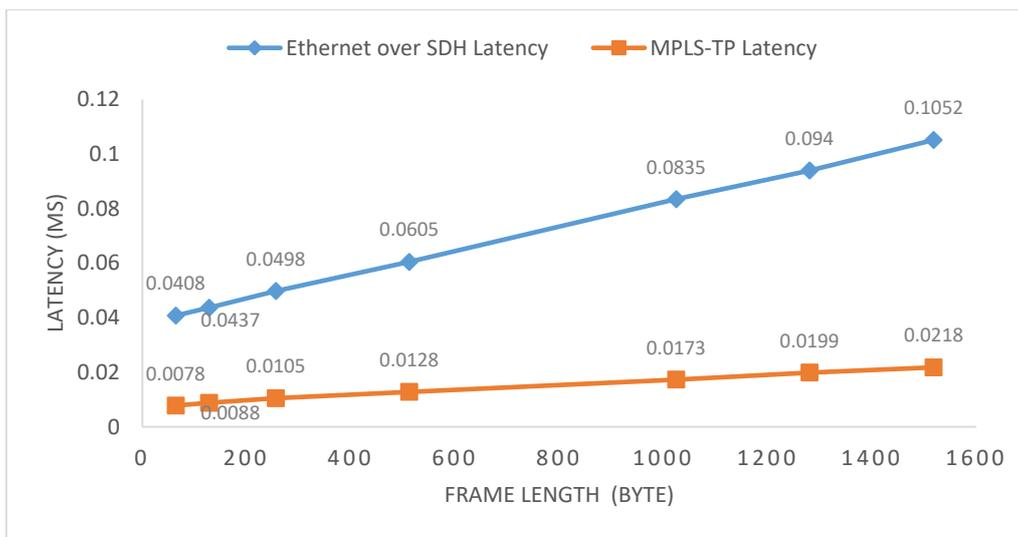
Figure 5. The Latency Values of Ethernet over SDH and MPLS-TP
