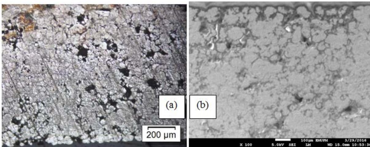
Figure 2. Micrographs of iron powder compact notched on the bottom surface (a) OM image (b) FeSEM image
