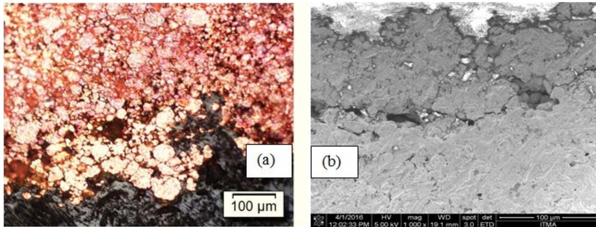
Figure 4. Micrographs of copper powder compact notched on the bottom surface (a) OM image (b) FeSEM image
