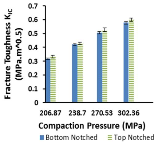
Figure 3. Variation of fracture toughness with compaction pressure for copper powder compacts notched on different surface
