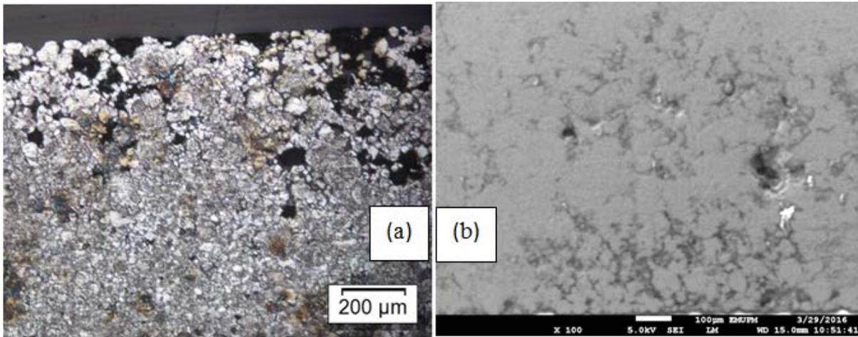
Figure 1. Micrographs of iron powder compact notched on the top surface (a) OM image (b) FeSEM image
