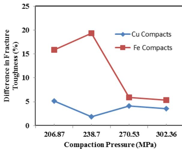
Figure 4. Percentage difference in fracture toughness at different pressures for iron and copper powders
