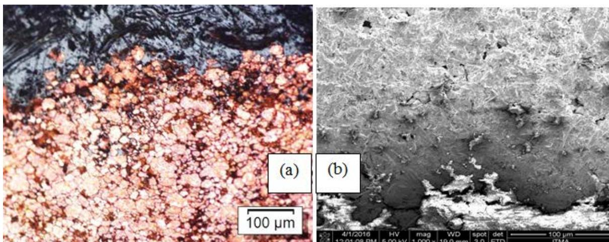
Figure 3. Micrographs of copper powder compact notched on the top surface (a) OM image (b) FeSEM image
