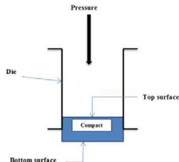
Figure 1. The top and bottom surfaces of a compact
