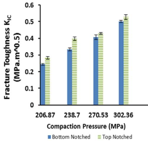
Figure 2. Variation of fracture toughness with compaction pressure for iron powder compacts notched on different surface
