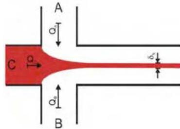
Figure 1. Schematic view of hydrodynamic focusing in a four channel intersection(Dziubinski 2012)
