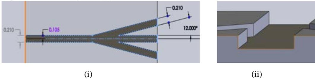
Figure 2. CAD design of the microfluidic channel (i) 2D profile (ii) step height of the design
