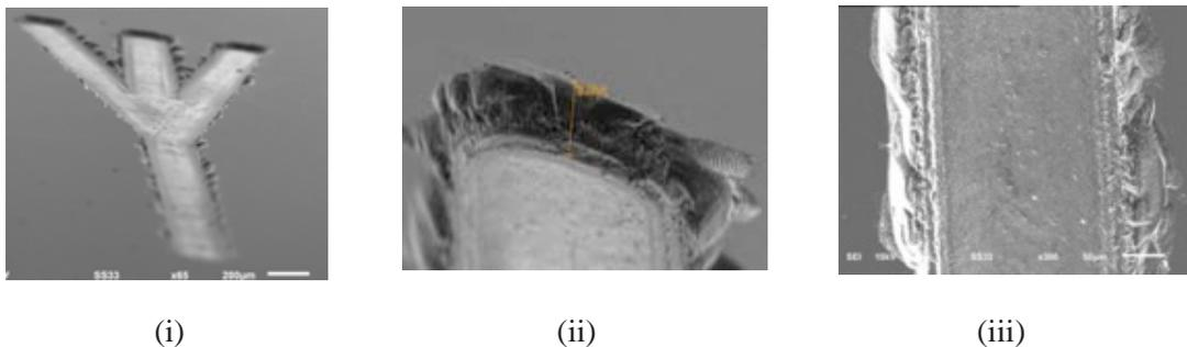
Figure 3. SEM images of machined micro surfaces for the fabricated micro channels with different magnification: (i) 65x (ii) 350x: step height (iii) 300x
